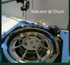
Use indicators to measure deflections and understand contribution of each of the major components with load cell inserted in place of springs.
