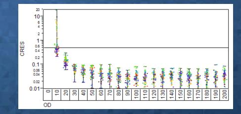
CRES[Ohms] vs. OD[um] FFI Internal Measurement
