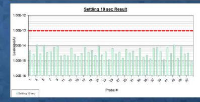
2D-MEMS & 3D-MEMS probe card both showed equivalent low electrical leakage performance
