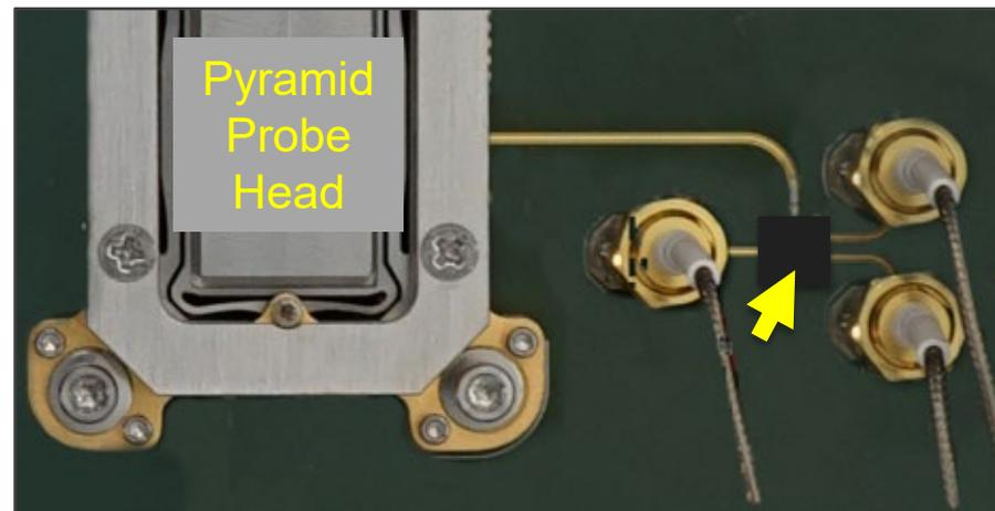
Full Path loss from Connector to probe tip including switch
