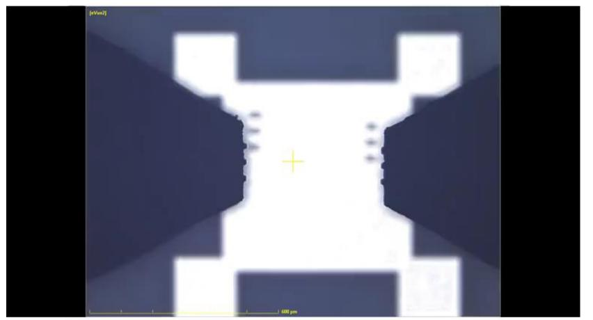
Probes grow as temperature goes from 25 to 125 and then shrink going to 25
