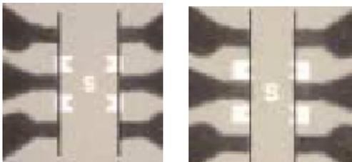
Proper amount of overtravel for calibration on Impedance Standard Substrates (ISS) can be set using alignment marks on the ISS.
