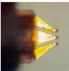
Always observe the probe tips when making the contact with the DUT. With the microscope focused on the DUT and the probe tips safely raised, the probe tips appear out of focus.
