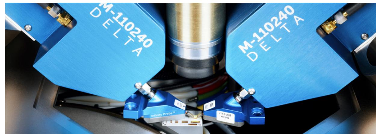
Load-pull measurement setup: FormFactor's Infinity probes are connected directly to the tuners. This minimizes insertion loss and maximizes Gamma. The setup integrates a high power microscope objective, enabling easy visibility of contact pads as small as 30  $\mu\text{m}$  with micron level accuracy. FormFactor's patented eVue Crash Detection protects your valuable equipment.
