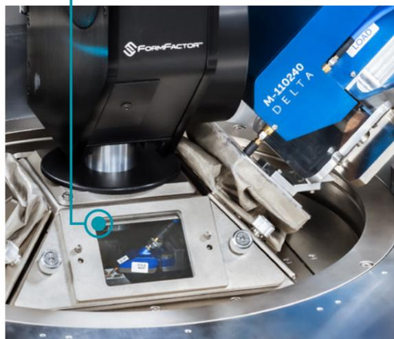
RF TopHat with I.T.O. coated window and patented FlexShield interface.
