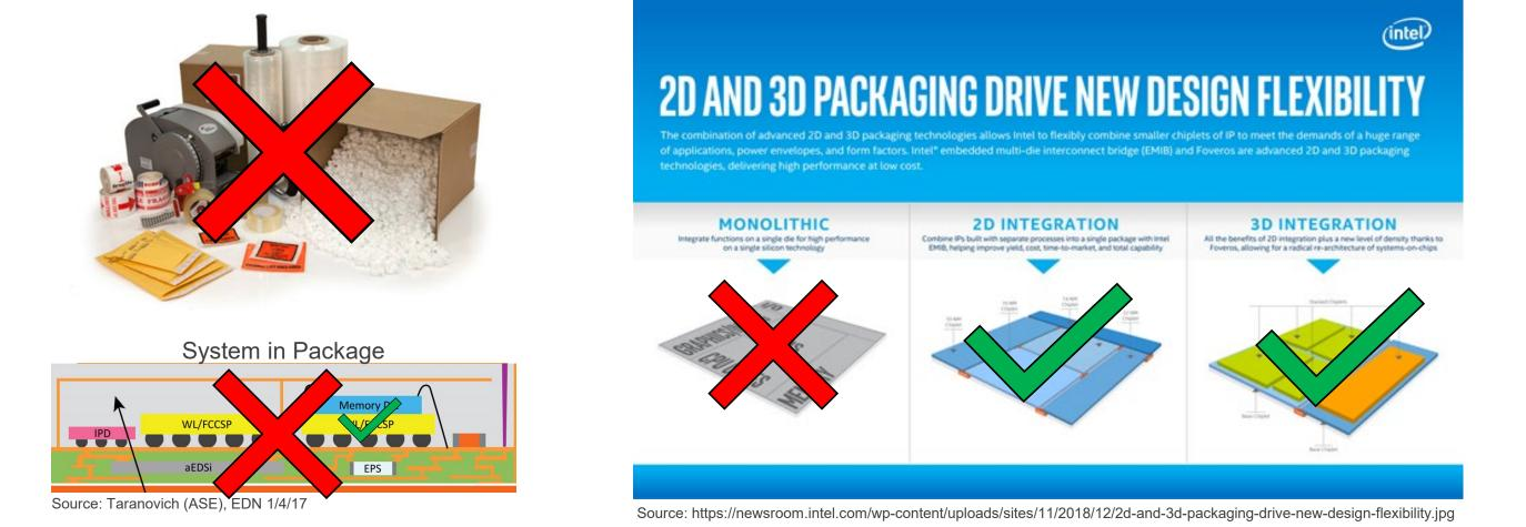
Advanced Packaging = Assembly of multiple die either directly to each other or through interfaces with interconnect densities and electrical performance comparable to that of the individual component die
