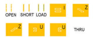
Fig. 9: Complete Set of Dual Calibration Standards
