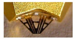
Fig. 2: CPW Contact Structure of a Dual IZI Probe 40 K3N GSGSG 150
