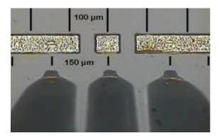
**Figure 7:** OPEN Standard and 150 µm GSG Probe
