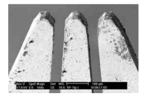
**Fig. 3** (source GFD Ulm): View of a GSG IZI Probe tip
