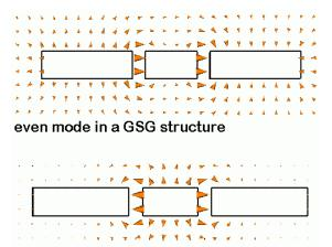
odd mode in a GSG structure Fig. 1: Even- and Odd-Mode in a CPW Structure
