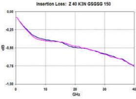
**Fig. 4:** Single Signal Insertion Loss of a Dual I**Z**I-Probe
