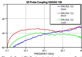
Fig. 5: Dual IZI Probe: Isolation between Both Channels
