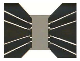
**Fig. 8**: LOAD standard on CSR 31, GSGSG 150 μm Pitch
