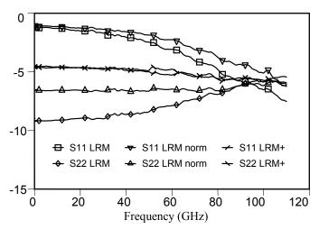
Fig. 6. Results of port symmetry verification for the LRM, the normalized LRM, and the LRM+ calibration using the RM 8130 series attenuator.
