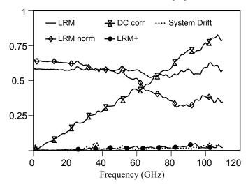
Fig. 5. The maximum possible differences between measurements of passive devices from NIST multiline TRL calibration for the simple LRM, the normalized LRM, the DC load corrected LRM+, and the complete LRM+ calibration.
