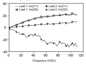
Fig. 4. The imaginary part of the measured port 1 (Z11) and port 2 (Z22) impedance of the load standard (Load 1) and a resistor (Load 2), located on the RM 8130.
