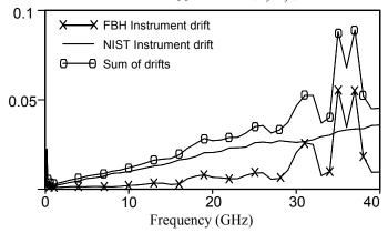
Fig. 1. Verification results on integrity of the wafer-level measurement setup used.
