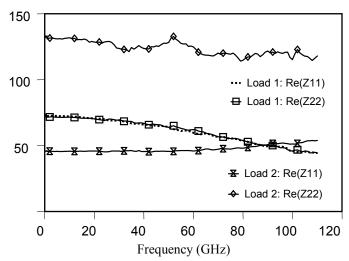
Fig. 3. The real part of the measured port 1 (Z11) and port 2 (Z22) impedance of the load standard (Load 1) and a resistor (Load 2), located on the RM 8130.
