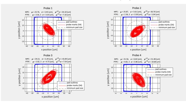
Measured data: 54 sets of die touchdowns / probe scrub marks, at multiple locations across 300 mm wafer, with accurate touchdown of 4 motorized probes on 30 µm pads, at 6 different temperatures ( 25, 150, -45, 175, -55, 200°C). Conditions include wafer soak 3 hr, die soak: 10 min, and 30 min contact test time.
