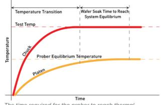
The time required for the prober to reach thermal equilibrium before probes can contact the pads is referred to as transition soak time or thermal soak time.
