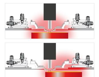
When the hot chuck is moved, a thermal imbalance in the prober is created.
