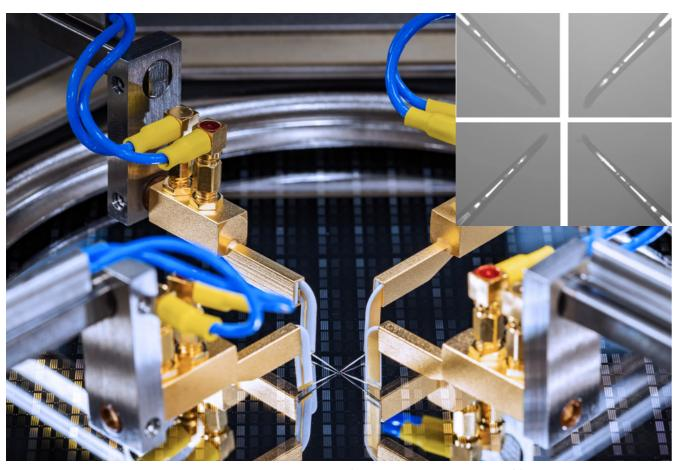
Advanced laser-marked probe needles enable highest accuracy for small pad probing down to 30  $\mu$ m.
