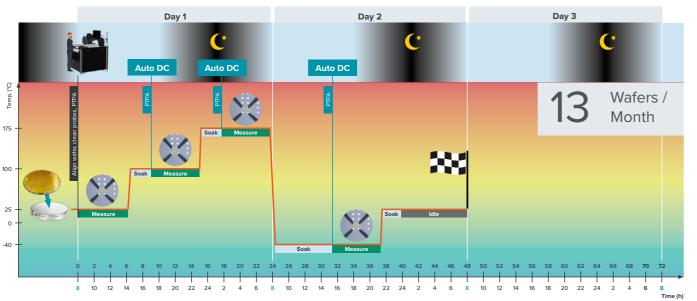
Figure 6: A FormFactor probe station with Autonomous DC Measurement Assistant achieves a 1.8X increased wafer throughput and requires 75% less test engineers time than Figure 5.\*
