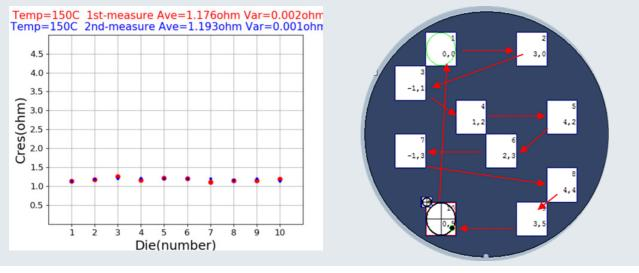
Consistent and low contact resistance measured on 10 dies across a wafer at 150°C. Average contact resistance is measured at 1.176  $\Omega$  with a variance of 0.002  $\Omega$  (first measurement) and 1.193  $\Omega$  with a variance of 0.001  $\Omega$  (second measurement).
