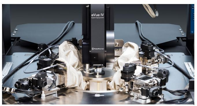
FormFactor's CM300xi-ULN Probe Station with Auto DC Measurement Assistant. The solution is also available for the CM300xi, SUMMIT200, Summit 12000 and Elite.
