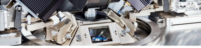
"Only the **Autonomous RF Measurement Assistant**, a combination of programmable positioners, a precise digital microscopy system and advanced pattern recognition algorithms, enables fully autonomous, hands-free calibrations and measurements of RF devices over multiple temperatures."
