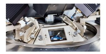
Reducing cable length to only 10 cm helps to improve system drift and dynamic range.
