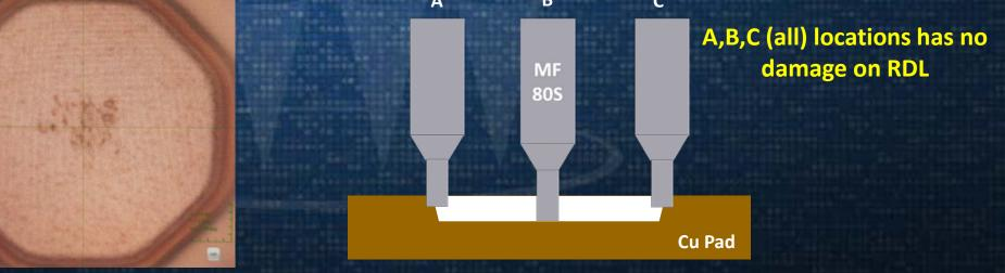
Contact Mark on Dummy Pad for Evaluation No broken tip issue at probing on the sidewall of pad SW Test Workshop | June 3-6, 2018
