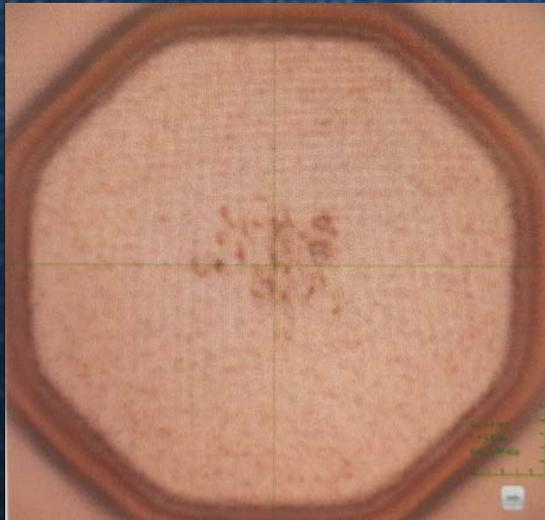
Contact Mark on Dummy Pad for Evaluation
