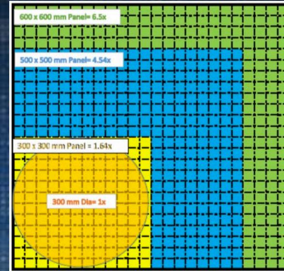
In comparison to 300mm FOWLP, alternative Fan-out Panel Level Packaging (FOPLP) provides larger processing area and lower cost per die
