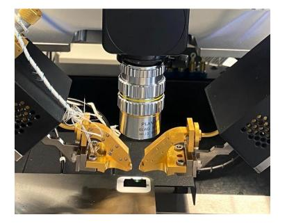
**Inclined Extender – 45deg WG - Probe**
