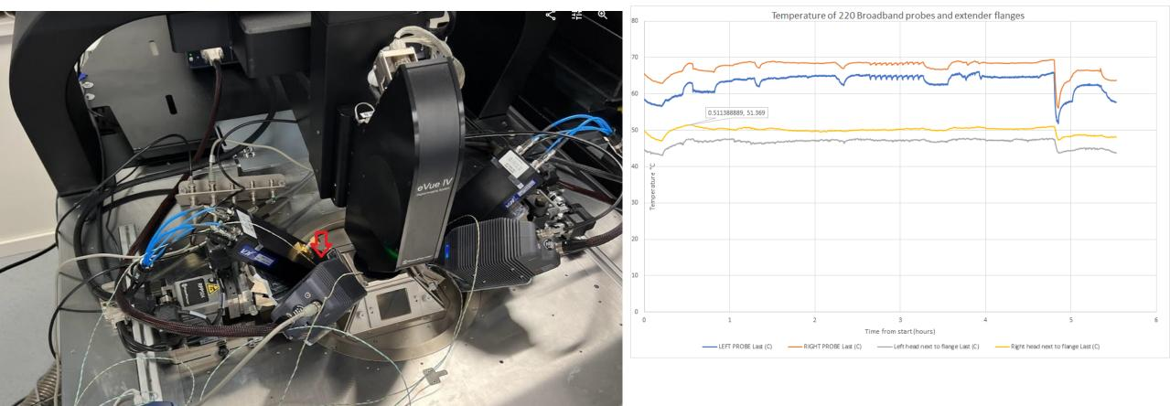
Probe tip at 150 °c but flange limited to 52 °c worst case and the rest of the extender is in ambient air with platen jet cooling
