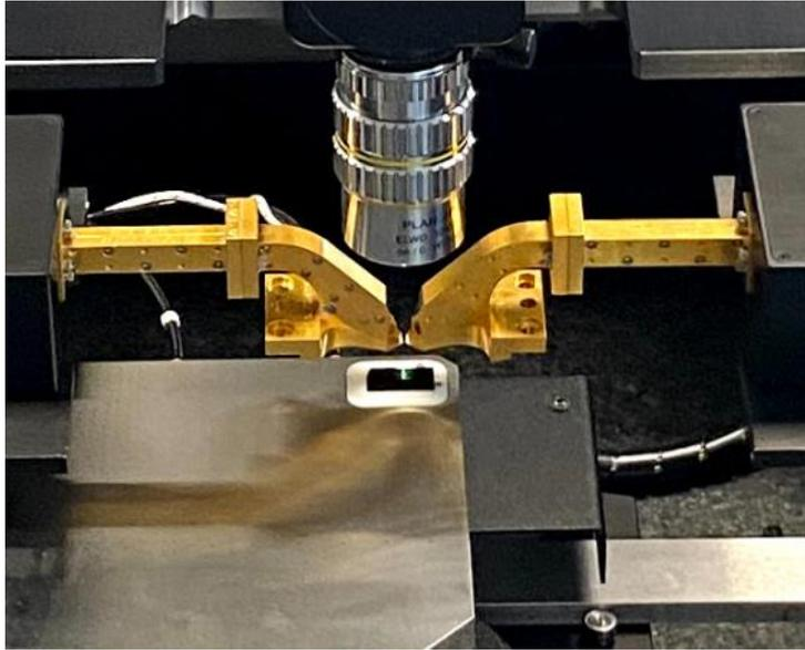
Horizontal Extender – 50mm VDI WG - Probe
