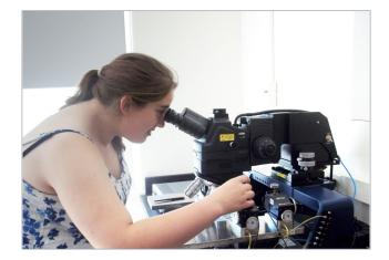
Figure 2: A student researcher operates a Cascade EPS150FA probe system to acquire data on the electrical behavior of newly synthesized materials.
