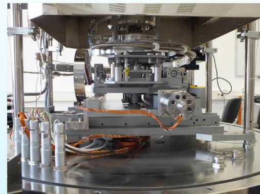
Cryogenic stage and radiation shield with an anti-reflecting surface towards the DUT
