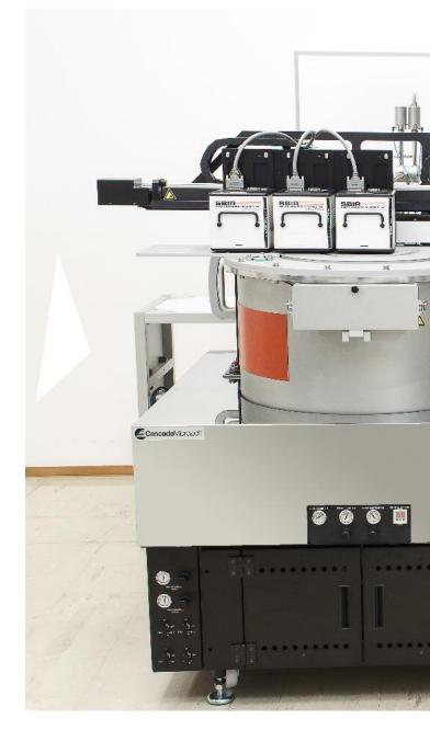
• For optimal cryogenic test, a cryogenic probe station is used to handle and thermalize the DUT, Wafer, multiple-samples, or
