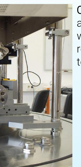
Cryogenic stage and radiation shield with an antireflecting surface towards the DUT
