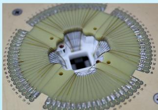
Cryogenic shielded cabling required to maintain signal integrity at temperature
