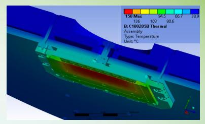
Thermal model of a probe card with prober chuck temperature set at 150°C
