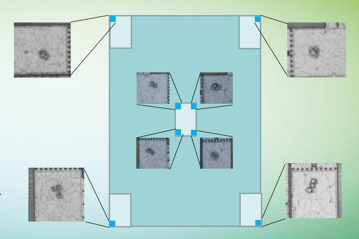
Architecture demonstrating very stable scrub mark placement from -40°C to 150°C
