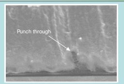
SEM images of pad damage issues causing device failures/issues
