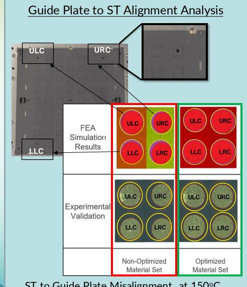
ST to Guide Plate Misalignment at 150°C
