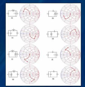
Complex impedance matching with discrete components
