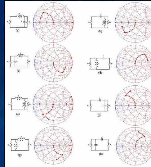
Complex impedance matching with discrete components
