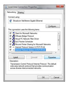
3. Select **Alternate Configuration** tab and click **User configured**. Type in the hardwired IP address you have selected. Repeat this step on the VNA if it is not already hardwired. Use those IP addresses to connect the two with a single LAN cable. If you have IT administrators, ask their advice on how to select IP addresses.
