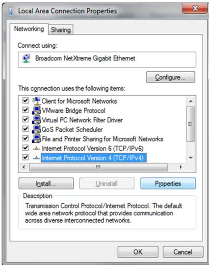
3. Select **Alternate Configuration** tab and click **User configured**. Type in the hardwired IP address you have selected. Repeat this step on the VNA if it is not already hardwired. Use those IP addresses to connect the two with a single LAN cable. If you have IT administrators, ask their advice on how to select IP addresses.
