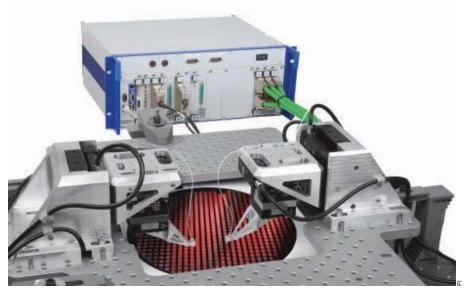
**Figure 2.** A fast multichannel photon alignment (FMPA) system for double-sided probing of on-wafer waveguide devices. Fully digital and closed-loop, it implements exclusion-zone capability, an internal data recorder, nanoscale-stable position-hold, and firmware-based fast scanning, modeling and multichannel  $N \times M$  gradient search capability.
