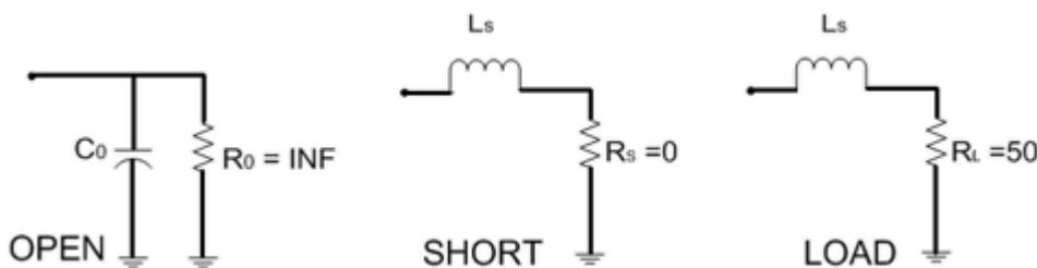
Figure 5. Parasitic elements
