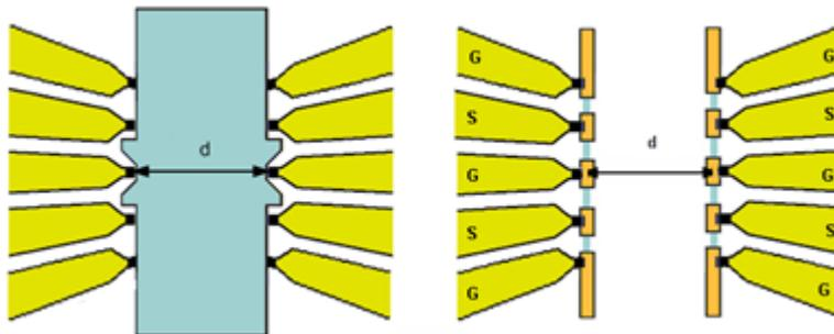
Figure 3. Probe spacing
