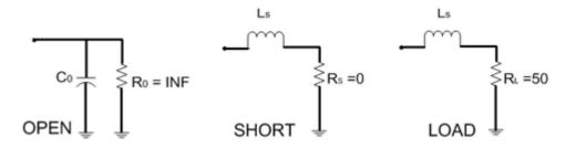
Figure 5. Parasitic elements
