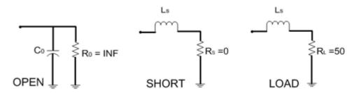
Figure 5. Parasitic elements
