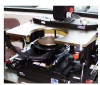
SQ-117-317-02 — 6-inch Gold Chuck Adapter, 0 to +200°C, w/Aux, Dovetail Mount
