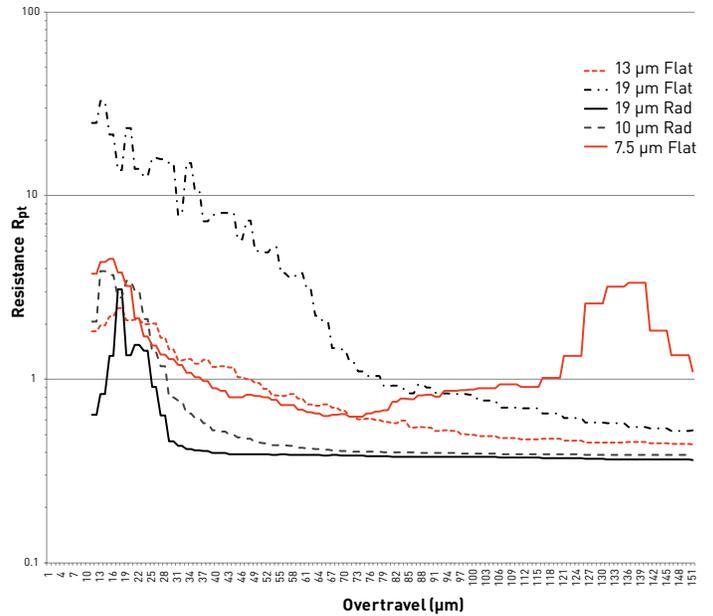
Figure 6. Results of probe resistance (probe tip + contact resistance).
