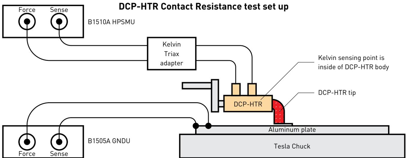
Figure 2. Electrical set-up used to measure contact resistance.
