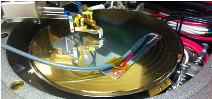
Figure 3. Test substrate with Kelvin connection and two probes tested simultaneously.
