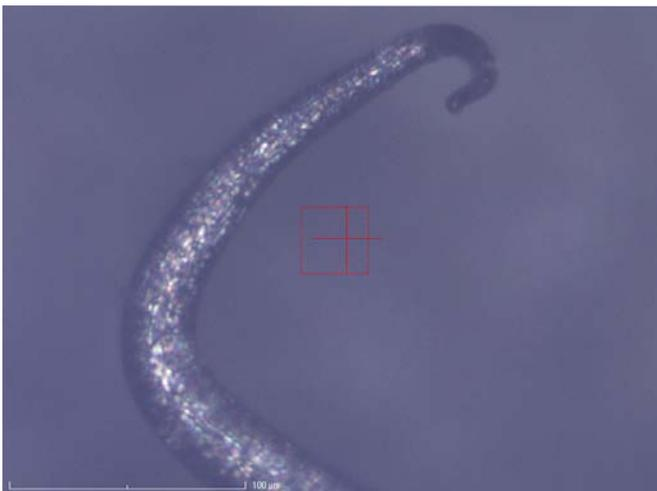
Figure 1 – A 'hooked' probe tip after excessive overtravel.
