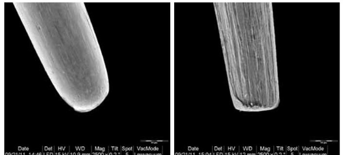
Figure 5. SEM Images showing the radius and flat probe tip shapes respectively.
