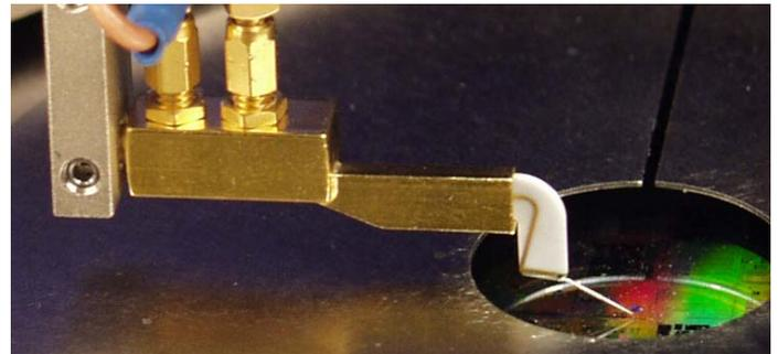
Figure 4. A DCP-HTR probe with probe needle.
