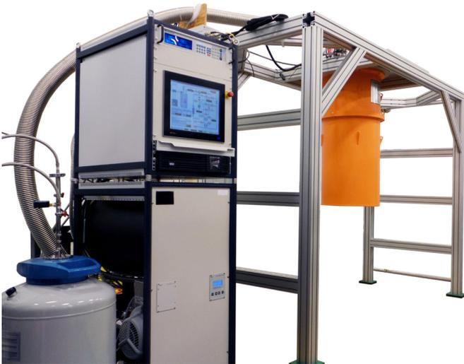
*FormFactor HPD LF-600 Cryogen Free Dilution Refrigerator*
