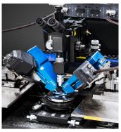
Universal mounting of frequency extenders from VDI for measurements up to 1.1 THz.
