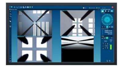
$\begin{tabular}{ll} \textbf{Multi-Camera Imaging:} Up to four simultaneous live views for accurate probe tip placement. \end{tabular}$
