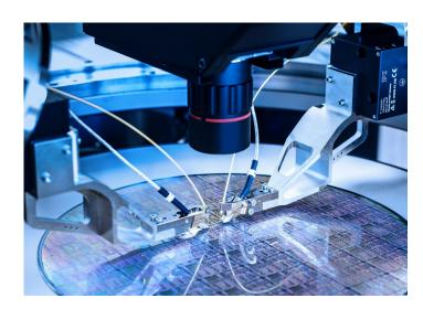
The new eVue V microscope on CM300xi with Autonomous SiPh setup
