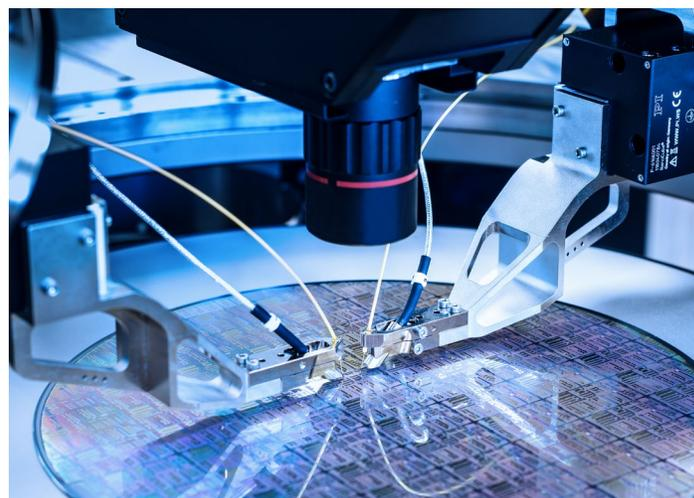
The new eVue V microscope on CM300xi with Autonomous SiPh setup
