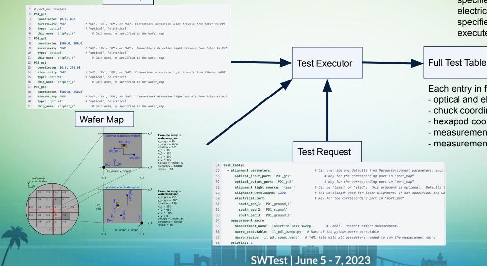
Wafer Map: Coordinates and dimensions of every subdie on wafer Port Map: Coordinates of every optical port (grating coupler) and electrical port relative to subdie origin Test Request: A table where each entry specifies a set of optical and/or electrical ports for a test site. It also specifies the measurement routine to execute and its parameters.
