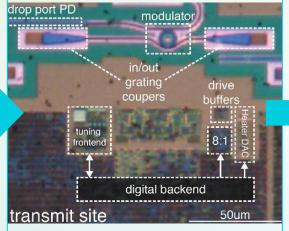
Dense integration of all electronics (TIAs, drivers, equalization, control) and photonics (waveguides, modulators, detectors) on a single CMOS chip
