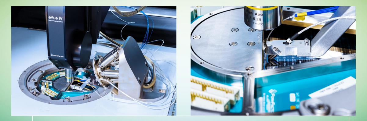
Fully Automated Wafer Level Co-Packaged Optics Electrical-Optical Probing
