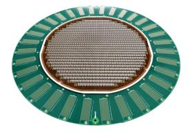
Genus Probe Card for Standard Test Cell Operation
