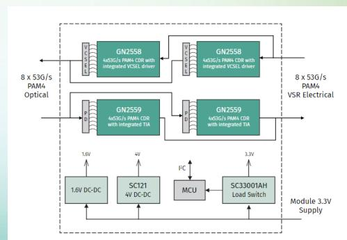
SEMTECH example 400G module that is part of an Active Optical Cable: https://www.semtech.com/applications/networkingcommunication/datacenters
