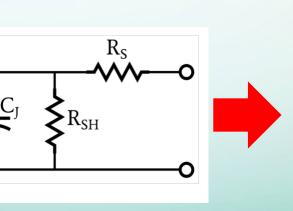
Photodiode equivalent circuit
