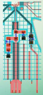
Photodiode emulating circuit
