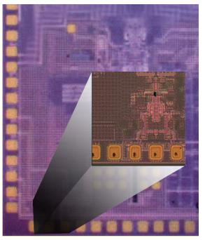
**FIGURE 1.** The automotive radar IC manufactured by DICE of Linz, Austria is  $80 \times 80 \mu m$  with up to 100 pads.
