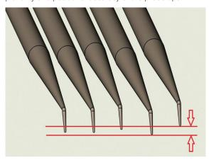
Figure 2. Conventional probe needles have planarity errors which cause excessive skate on the first probe to contact the pads.
