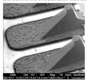
**Figure 3.** InfinityQuad probe tips manufactured by FormFactor are formed with a photolithography process and can be as small as  $8 \mu m$  long and  $12 \mu m$  wide.
