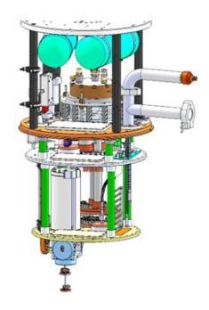
HPD Model 106 Rapid Cool Cryostat option and additional connector box
