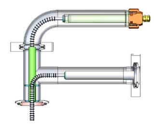
Rapid Cool Transfer Tube Receiver (top) and Outlet (bottom)
