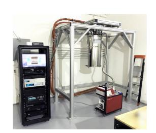
Model 119 Overhead Stand. Dimensions: 1.5m width, 1.23m depth, 2.21m inside height, 2.69m total height
