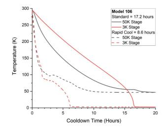
Cooldown time graph for a Model 106, with and without Rapid Cool
