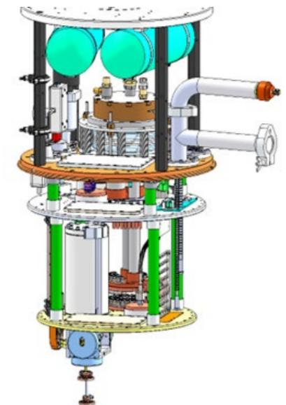
HPD Model 106 Rapid Cool Cryostat option and additional connector box
