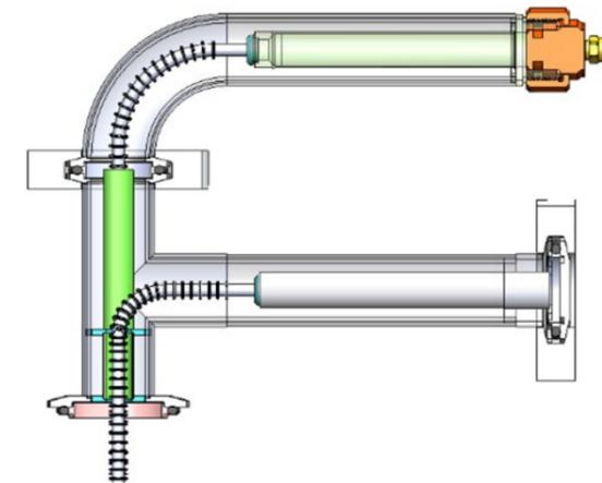
Rapid Cool Transfer Tube Receiver (top) and Outlet (bottom)
