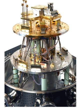
HPD Kilimanjaro 125 chip-scale semi-automated 4 K probe station with vibration isolation
