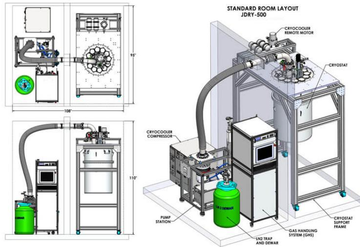
Standard Room Layout for Model JDry-500 Dilution Refrigerator
