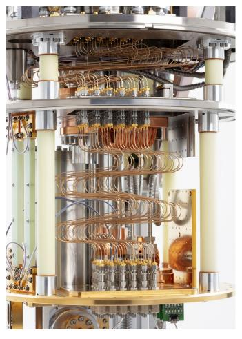
Close-up of HPD Model 106 ADR Cryostat
