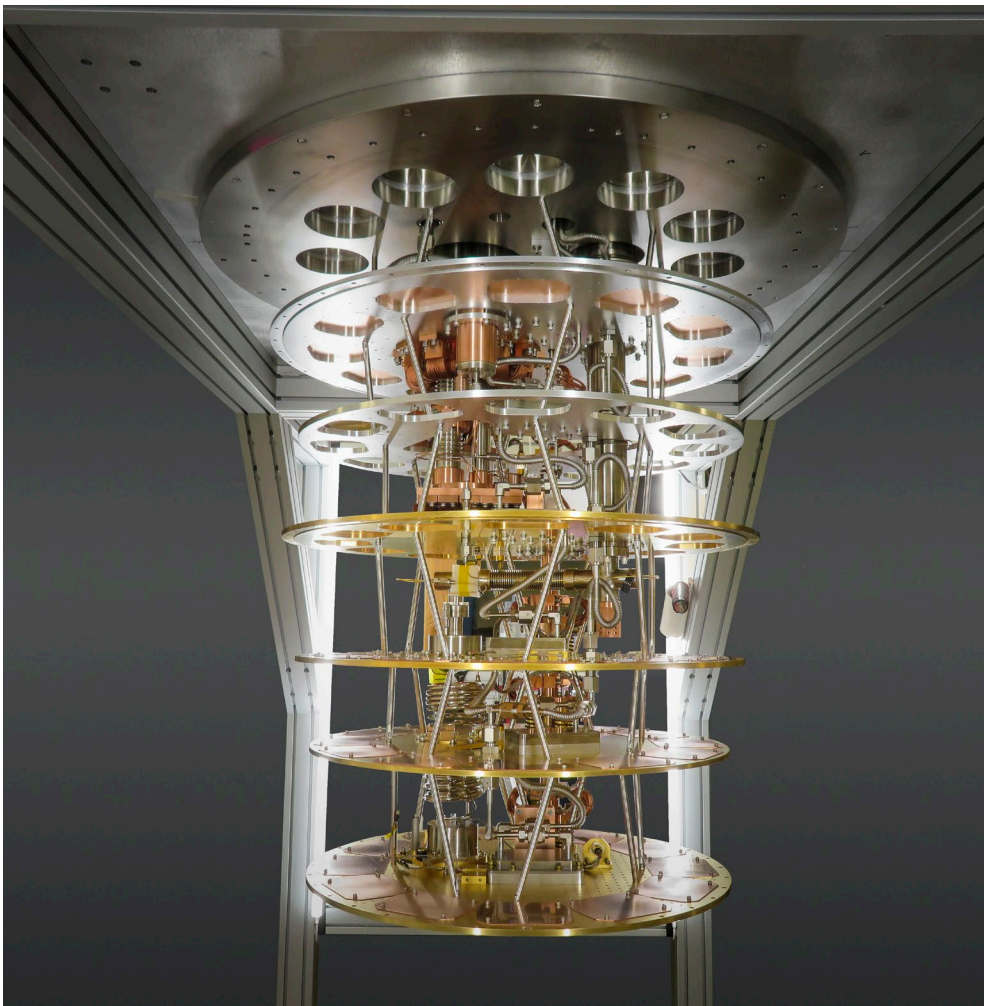
Aspect DR core with laser-weld heat exchangers provide high reliability with best-in-class cooling power and He3 efficiency.
