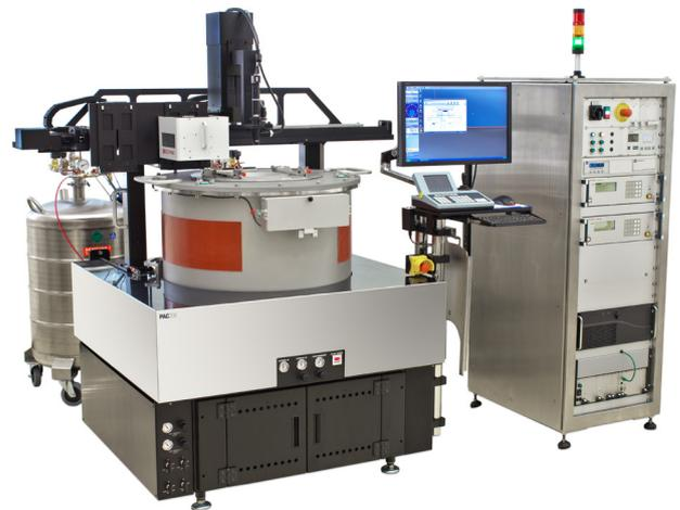
*PAC200 Semi-Automated Cryogenic Wafer Prober
