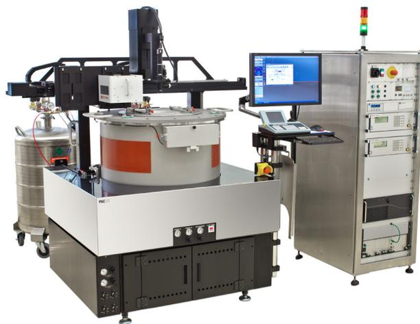
*PAC200 Semi-Automated Cryogenic Wafer Prober
