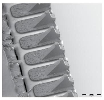
Uniform, tight-pitch contacts of InfinityQuad probes offer a parallel microscrub action with no side skate.
