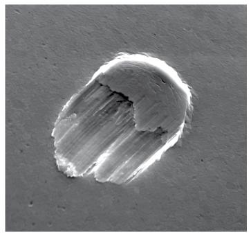
InfinityQuad probe mark on AI pad. Total damage window is typically W12  $\mu m$  x L15  $\mu m$  with scrub.
