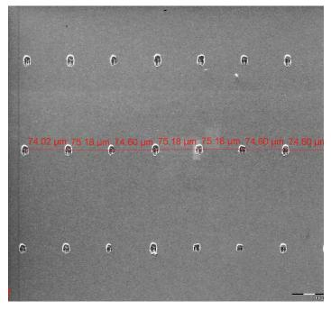
SEM images showing InfinityQuad tip-to-tip positioning accuracy <1  $\mu m$  at ambient.
