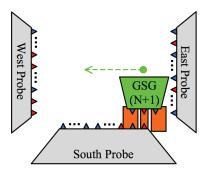
(d) Replace North probe with the N+1'th GSG probe and measure all thru pairs with ports in South Probe. Remount North probe afterwards.
