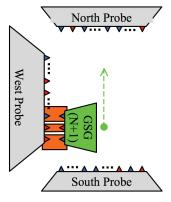
(e) Replace East probe with the N+1'th GSG probe and measure all thru pairs with ports in West Probe. Remount East probe afterwards.
