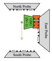
(c) Replace West probe with the N+1'th GSG probe and measure all thru pairs with ports in East Probe. Remount West probe afterwards.
