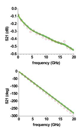
Fig. 6. Post-calibration measurements of a symmetric lossy transmission-line; using conventional 2-port SOLR calibration (thick green line) and using the presented N+1-port SOLT (red circle) / SOLR (blue circle) calibration.
