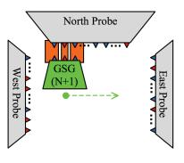
(b) Replace South probe with the N+1'th GSG probe and measure its SOL and all thru pairs with the ports in North Probe. Remount South probe afterwards.
