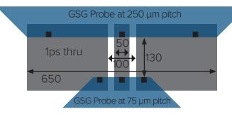
Figure 2. Dimensions of the 1 ps thru standard in ISS P/N 101-190 (units in  $\mu$ m).
