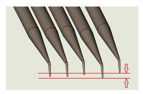
Figure 4. The planarity (first-to-last contact) can cause the first probe to skate off the pad by the time all probes have made contact.
