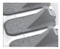
Figure 11. Small lithographically-fabricated contacts of Infinity Quad with a width of 12 μm and a contacting length of ~ 8 μm.
