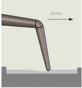
Figure 5. The more over travel applied the more skate occurs. The smaller the ratio, the more skating effect is suffered by excessive overtravel.
