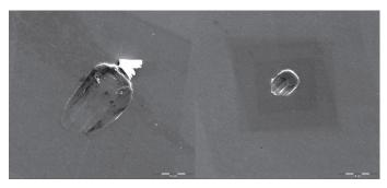
Figure 14. A good example of a conventional probe mark compared to an InfinityQuad probe mark using a similar scale.
