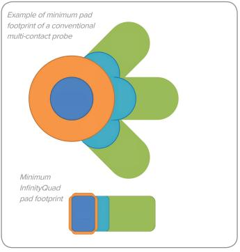
Figure 15. Including an error margin for automatic probing over temperature, the recommended pad area for InfinityQuad is five times less than conventional probes.
