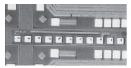
Figure 2. Probe pad structures within scribe street.
