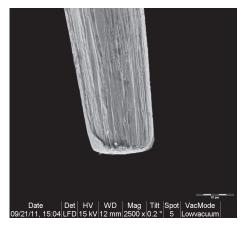
Figure 3. SEM image of a conventional DC probe contact area with a diameter of 19 μm.
