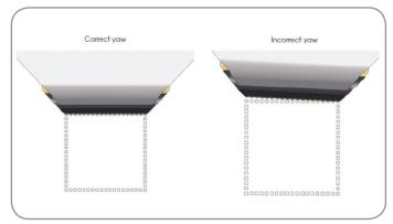
Fig 8. Effect of incorrect yaw alignment
