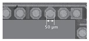
Figure 1. Small 50 µm pads of a semiconductor IC.
