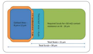
Figure 13. Footprint of the InfinityQuad probing budget uses 1/10 of the surface area compared to a conventional probe.
