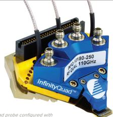
Figure 10. InfinityQuad probe configured with mixed DC, 20 GHz RF and 110 GHz mm-wave channels.
