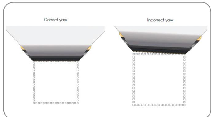
Fig 8. Effect of incorrect yaw alignment
